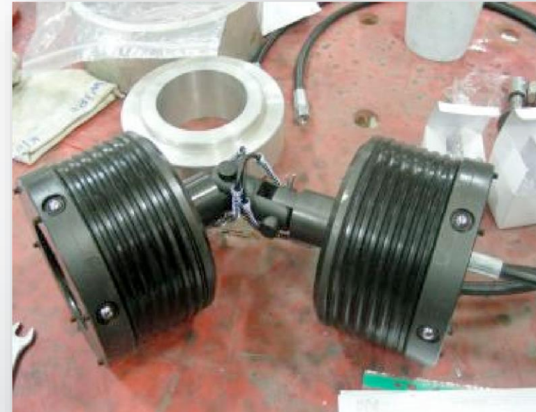
6" Flexi Tester – Riser isolation and weld testing
