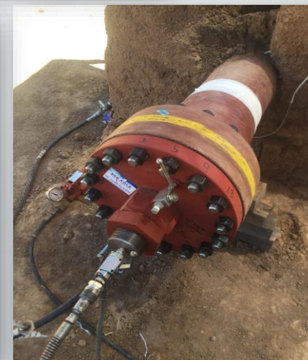
10" Flange Tester performing hydrotest on GRE pipe
